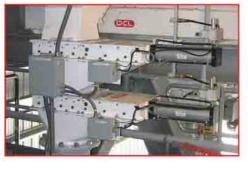
Blade seals are selected according to the material being handled and are available to suit any application. A molded urethane inlet liner provides an ideal blade seal when handling granular products. Additional frame seals are available and should be used when handling fine dusty material. Adjustable seals are also available to virtually eliminate the need for seal replacement. These seals are adjusted from the outside of the valve frame, which makes it unique to the industry.
